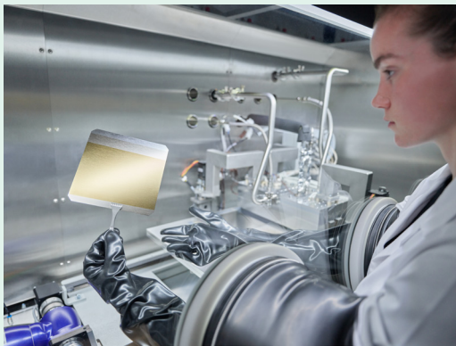
Figure 12. A spatial ALD tool equipped with glove box to deposit high quality \text{SnO}_2 films.
